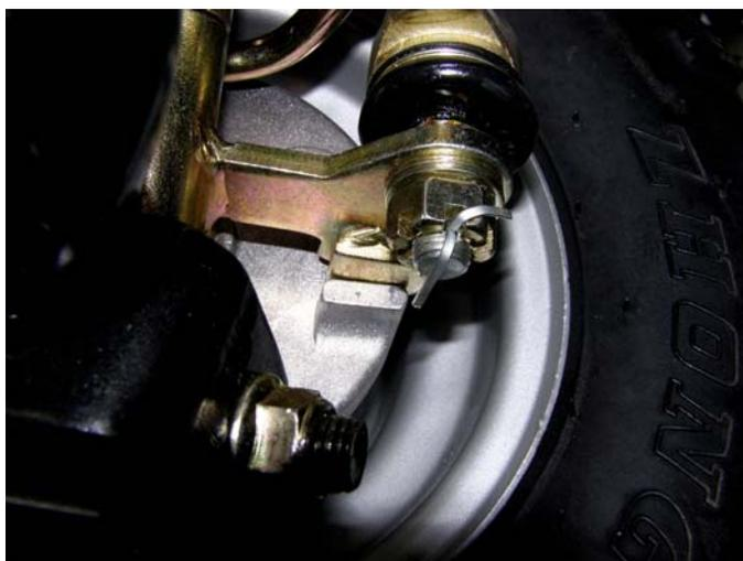
Make sure brake backing plate locator is in place before tightening wheel nuts.
